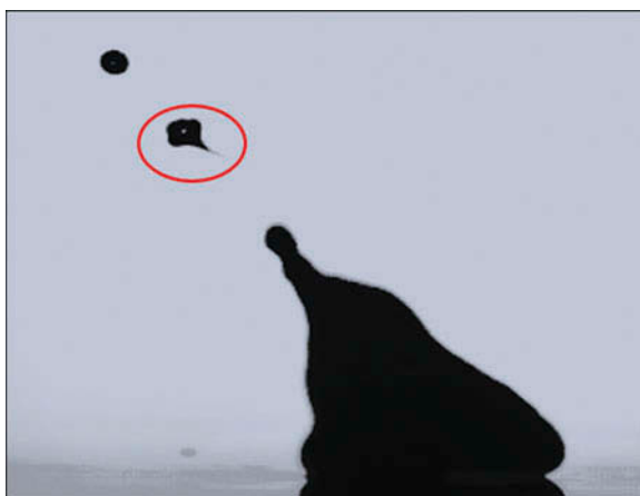
Figure 12. Puffing of a child droplet of 0.5681 mm ejected from parent droplet of Ø2.6 mm.
